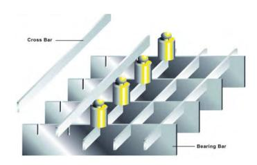
The SA Series press locked bar type is unique in appearance, high in load capacity, and is one of the most widely used aluminum swaged gratings. The cross bar is inserted in the notches of beaing bar and press locked into a stable structure at a force of 500 tons.
